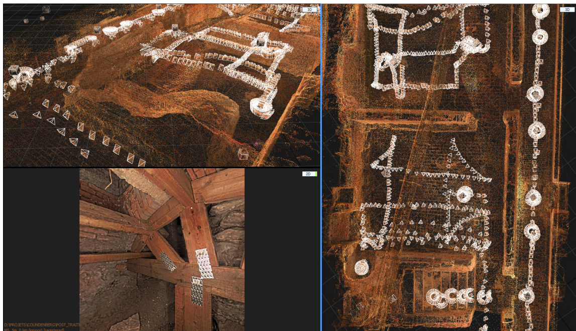
Figure 17. Registration of different photos with laser-scanning data. In white, the different positions of the pictures.
