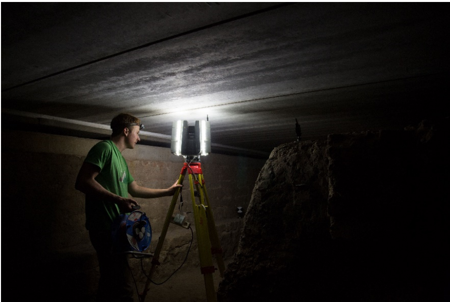
Figure 25. On-site acquisition with an adapted system to reduce problems in low-light conditions.
